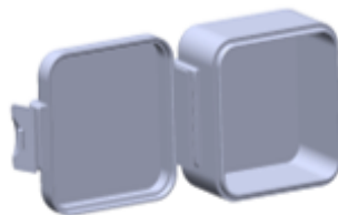
Fig. 5. Living hinge box for SLS printing machine.
