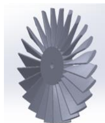
Fig. 4. Turbine blade for SLA printing machine.
