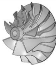
Fig. 6. Compressor wheel for SLM printing machine.
